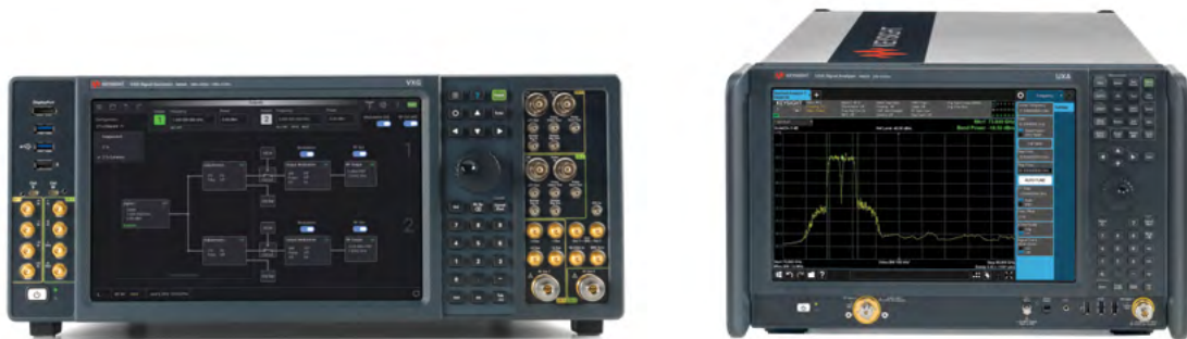
Figure 18.1. This configuration of the 5G R&D Test Bed supports 3GPP NR signal creation up to 44 GHz (lower left) and includes benchtop spectrum analysis up to 50 GHz (right), both with integrated 1 GHz bandwidth
