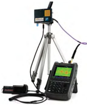
Keysight FieldFox handheld analyzer integrated with a phased array antenna
