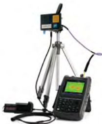
Figure 25.8. FieldFox phased array antenna coverage test system
