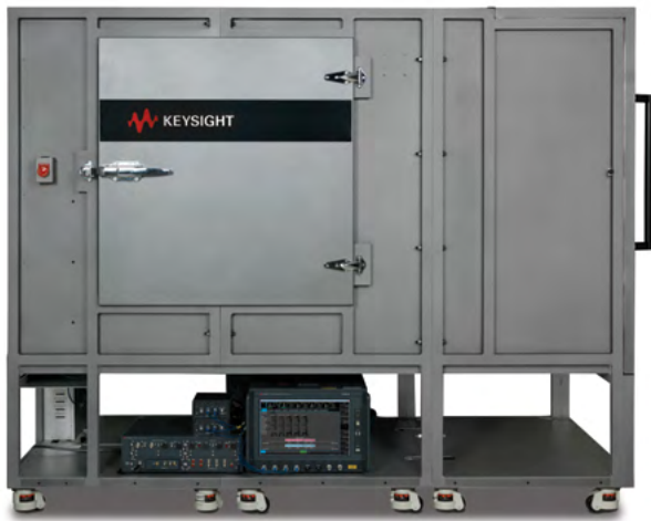
Figure 5.3. IFF CATR method for 5G mmWave OTA testing
