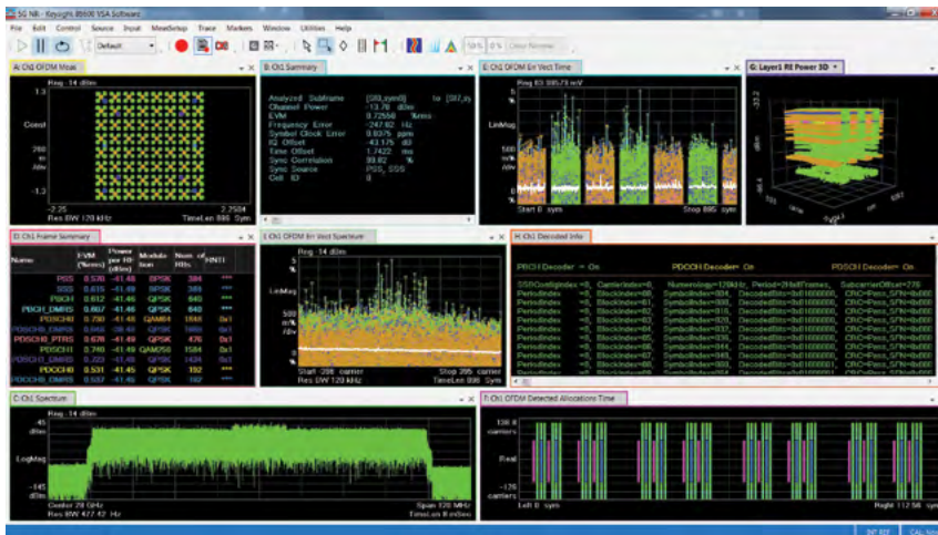
5G new radio modulation analysis PathWave 89600 VSA software (option BHN)
