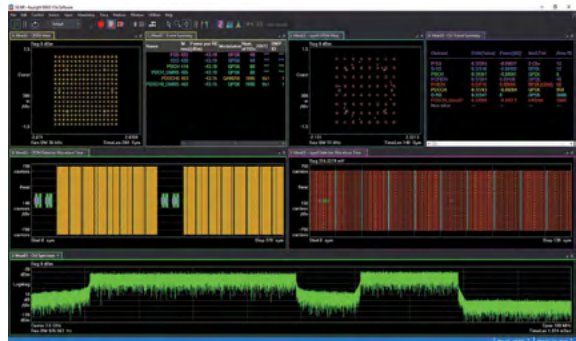
Figure 2.7. Using 5G signal generators, signal analyzers, and PathWave VSA software to analyze 4G and 5G waveforms
